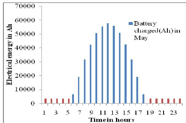
Figure 7: Variation of battery charging and discharging for the month of May
