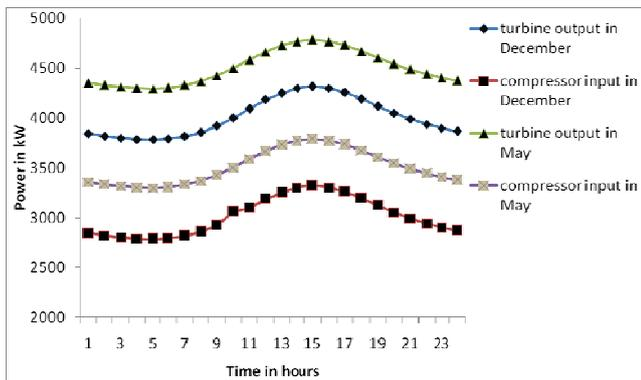
Figure 5: Variation of turbine power and compressor power
