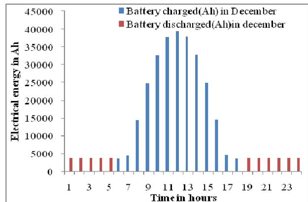
Figure 6: Variation of battery charging and discharging for the month of December
