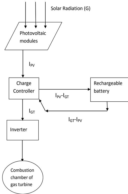
Figure 1: Schematic view of photovoltaic system
