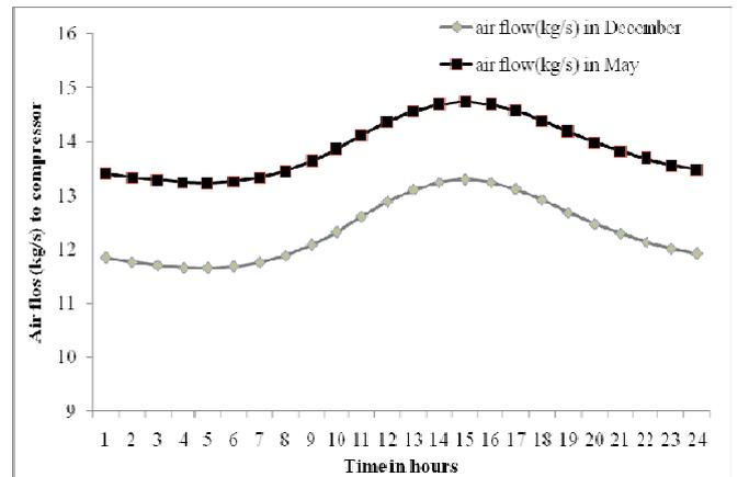
Figure 4: Variation of air flow rate(kg/s)to compressor
