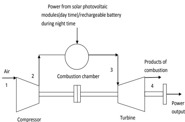
Figure 2: Schematic view of gas turbine operated by solar photovoltaic modules
